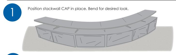
Screw 2½" deck screws to secure cap to block.
